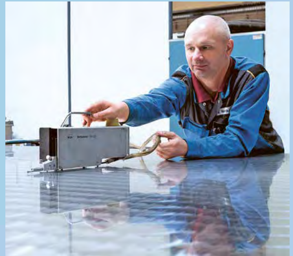
Checking the hot platens in production
