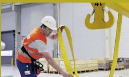
The 28-meter long part has to be secured and fastened every four meters
