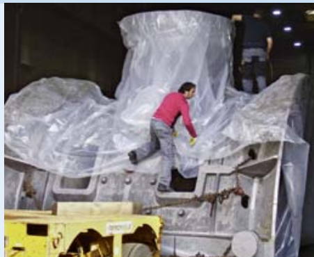
The gigantic housing section of a steam turbine made from nodular cast iron, 55 t, goes on a journey, carefully packaged...
