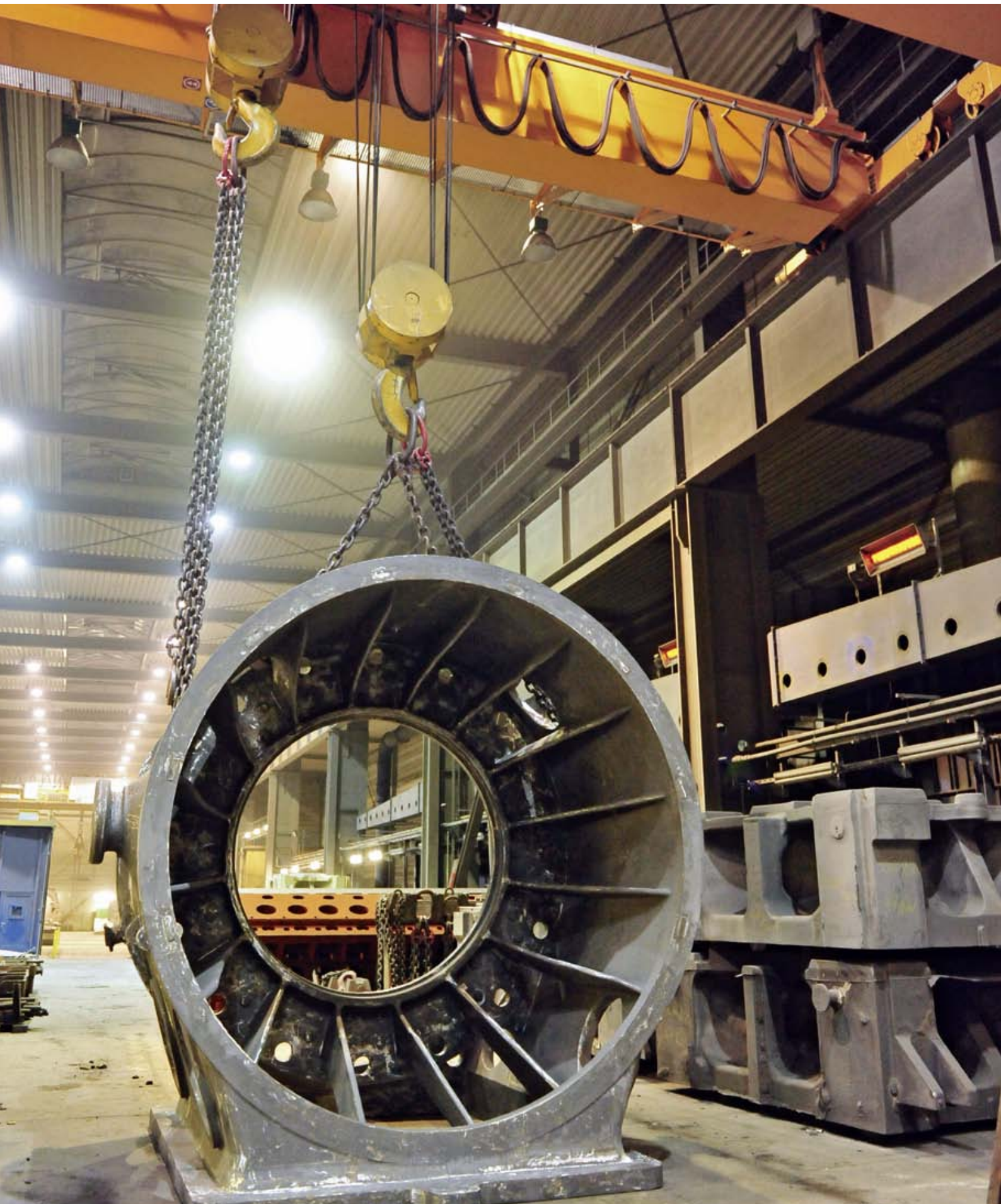
Fettling work: a housing for an underwater turbine
