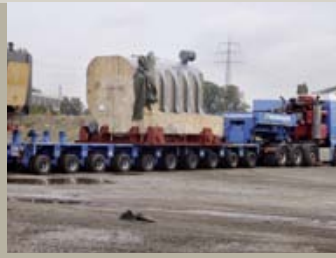
Transport of a table segment
