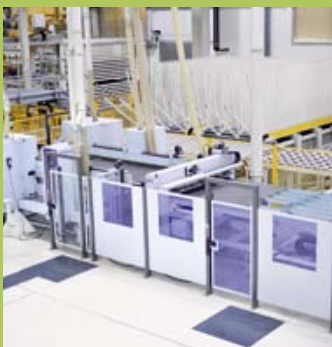
Cutting to size of finished boards
