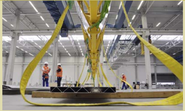
Long parts up to 28 meters in length can be moved quite easily by the crane
