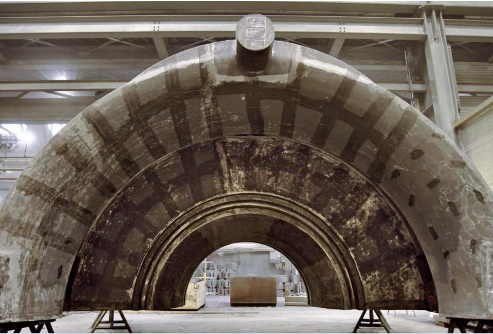
A steam turbine housing section, approx. 55 t, at the preliminary ultrasound test
