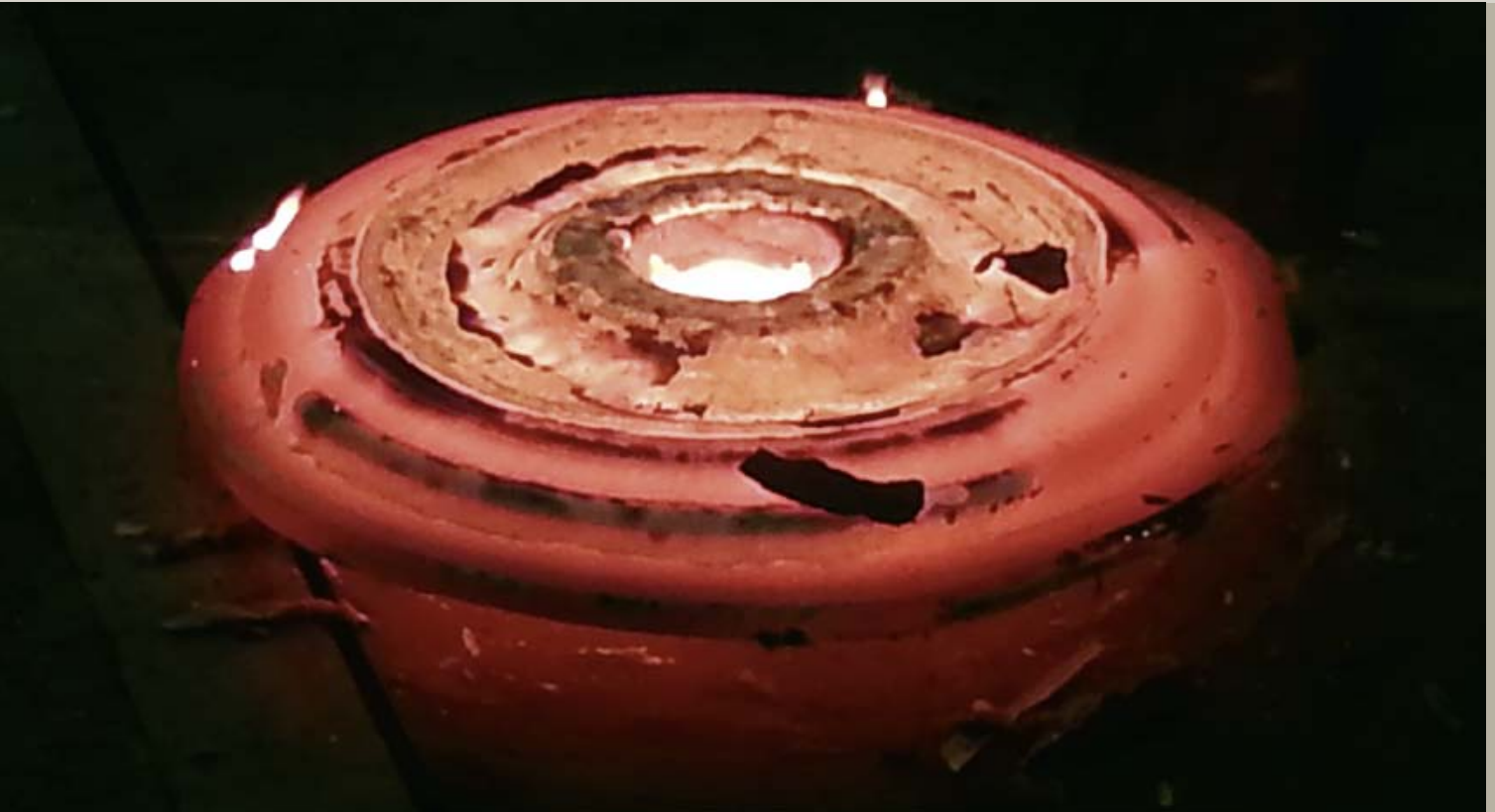
Product of the closed-die forging press for further processing on ring-rolling mill (test phase)
