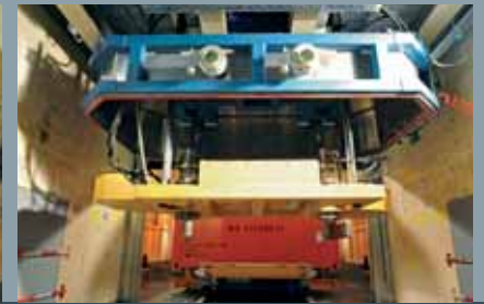
Concrete filling device for comminution and packaging of the heavy concrete segments of the biological shield
