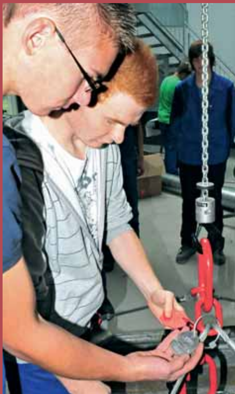
Synchronizing of the load-bearing capacity and the spread angle in accordance with the manufacturer's plate
