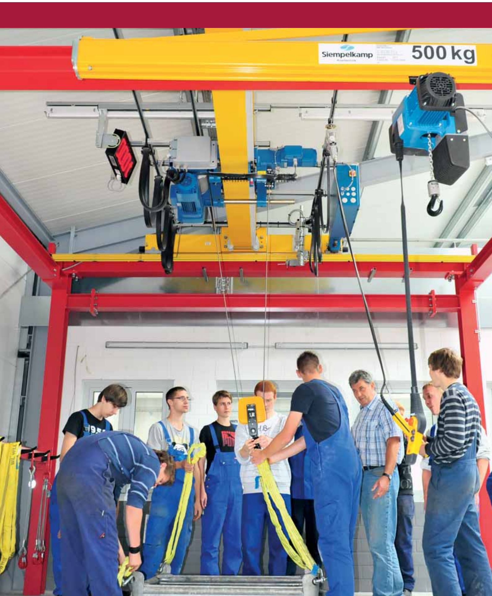
Training crane system: Trainees learn the professional and safe fastening of loads and the operation of a crane system
