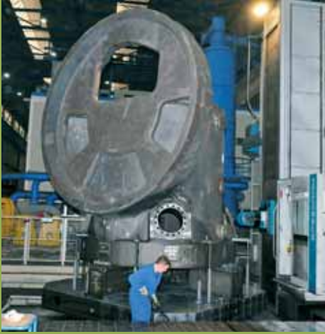
Machine carrier on a drilling machine
