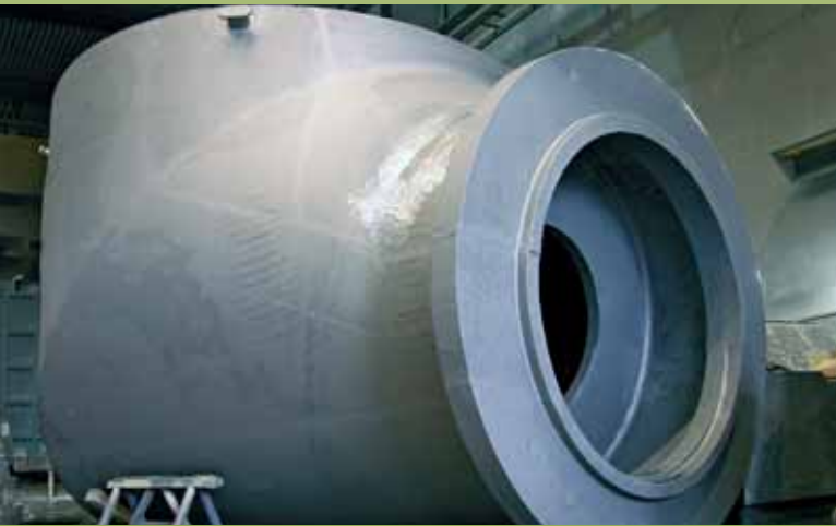
Machine carrier for 7.5 MW onshore wind turbines
