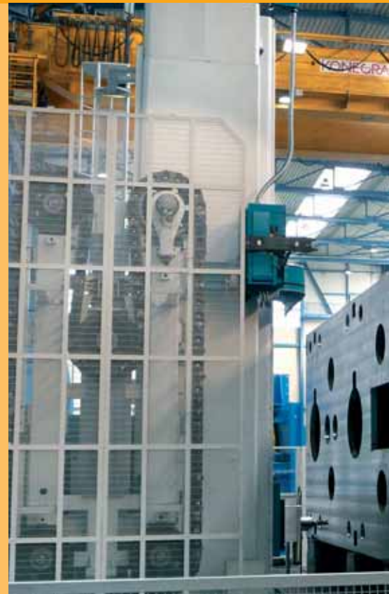
A press crossbeam under machining
