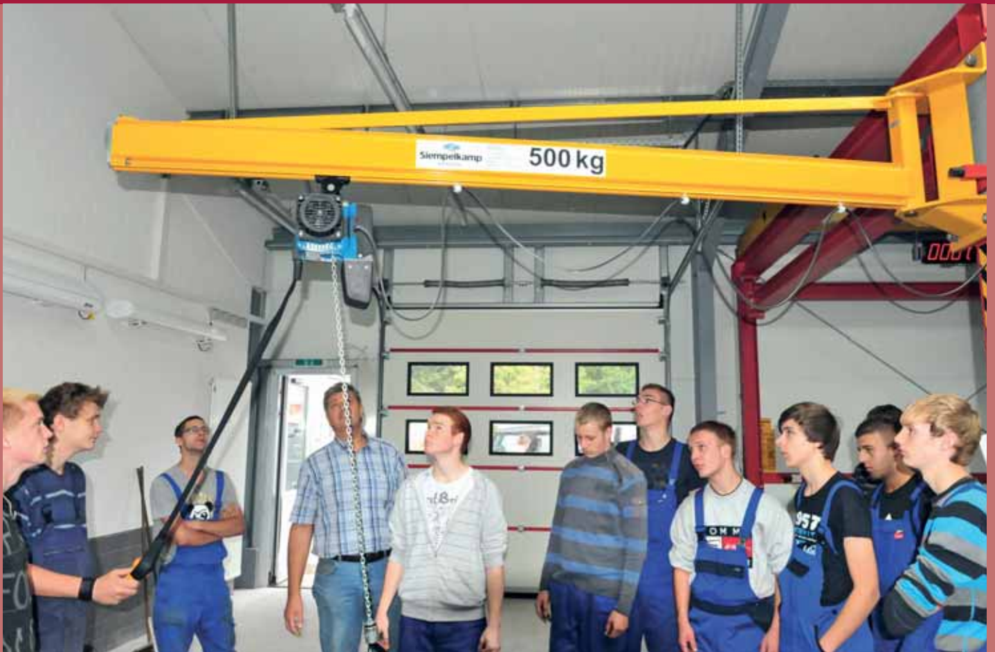
The slewing crane, a further component of the training crane system
