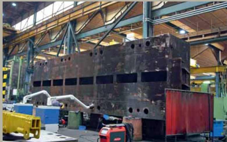
Lower crossbeam of the press in the welding shop
