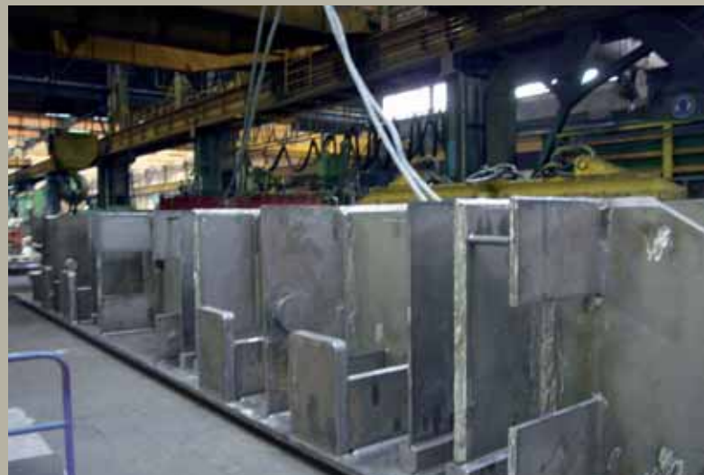
Moving crossbeam as welded construction
