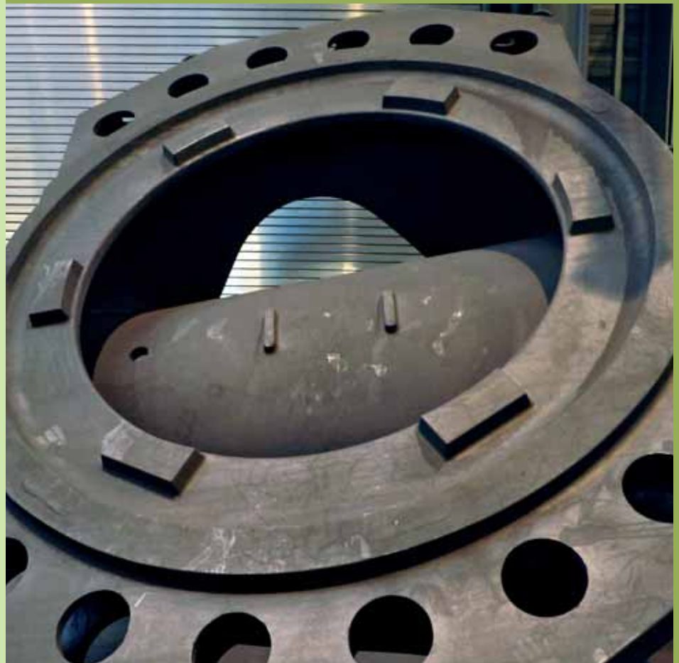
Machine carrier of a wind turbine
