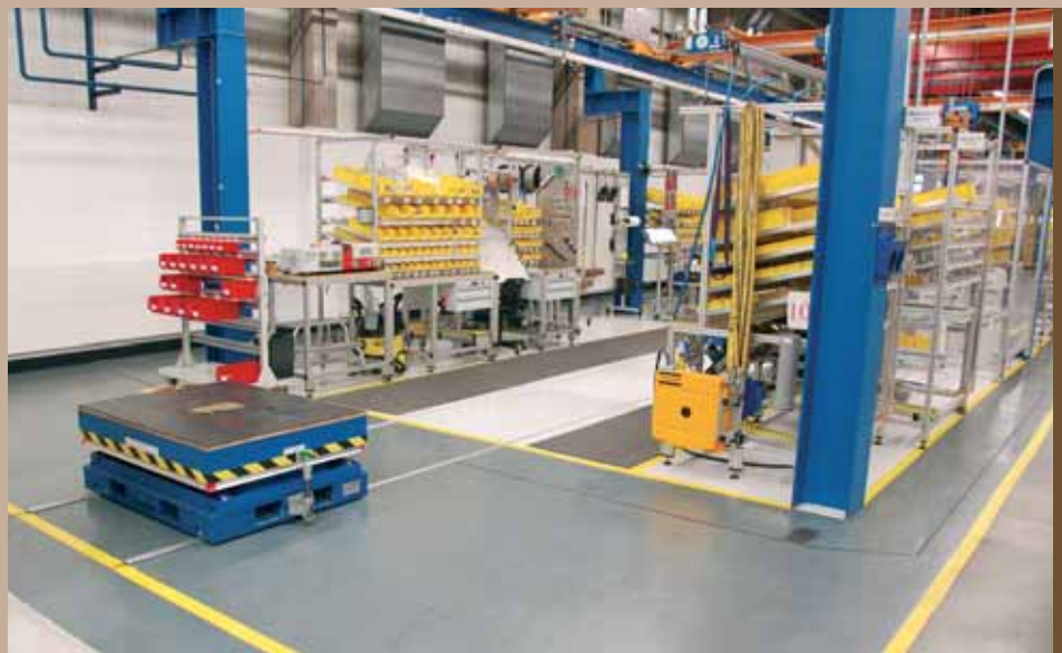
End of the assembly line, the trolleys are picked up by a forklift and transported back to the beginning
