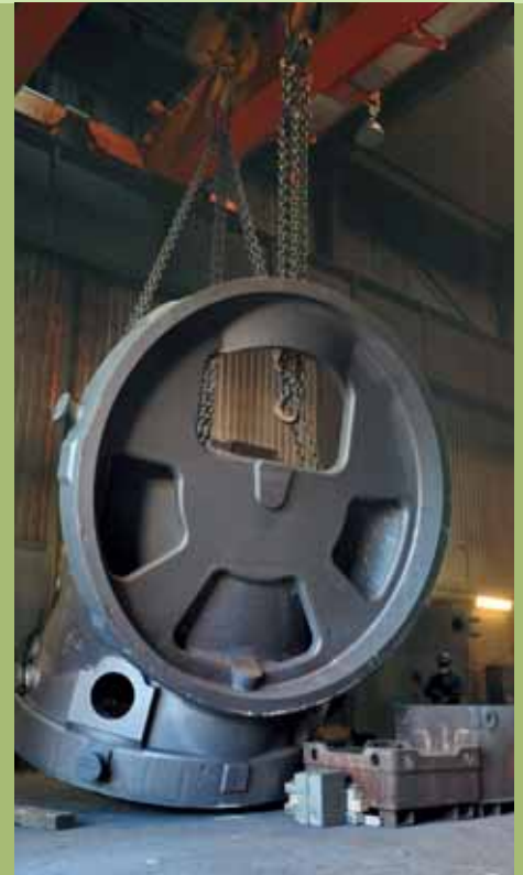
Areva machine housing in the fettling shop
