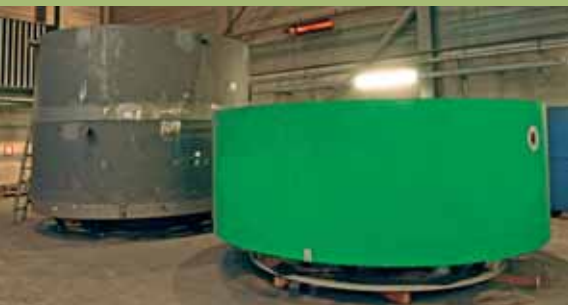
Areva component lower deck – bottom: view into lower deck during the ultrasonic testing for quality assurance
