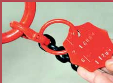
Synchronizing of the load-bearing capacity and the spread angle in accordance with the manufacturer's plate
