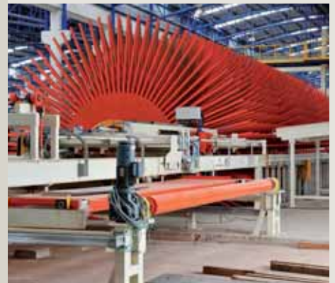
Cooling and stacking
