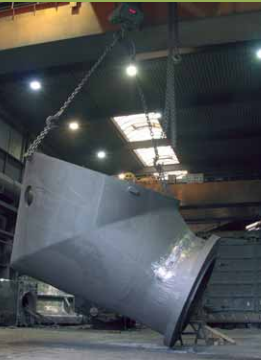
Machine carrier for 7.5 MW onshore wind turbines
