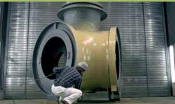
Rotor hub in the coating process
