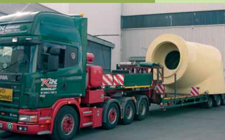
From left to right: transport of a 46 t machine carrier and a 36 t rotor hub
