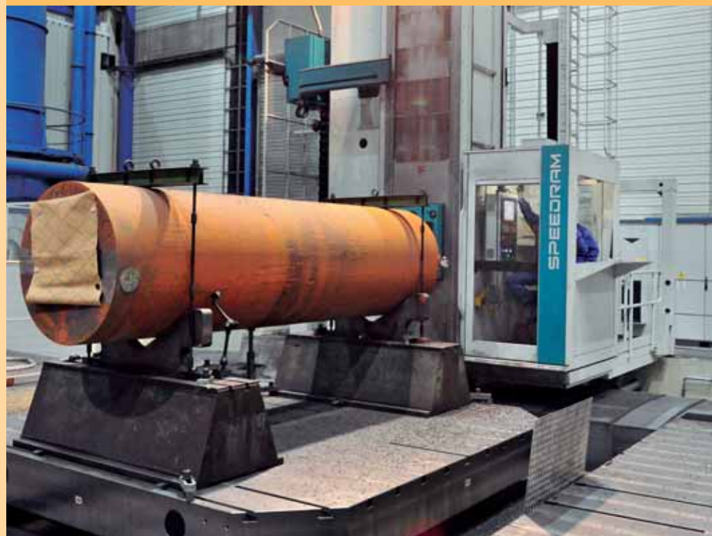
Milling of a cylinder component
