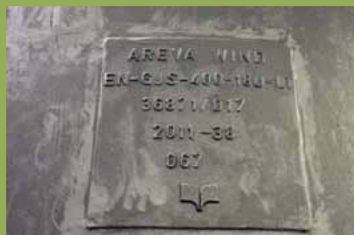
Type plate on an Areva Wind cast component, indicating the cast material and Siempelkamp casting sign among others
