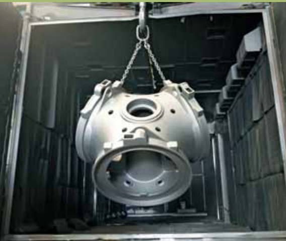
Rotor hub in the blasting shop
