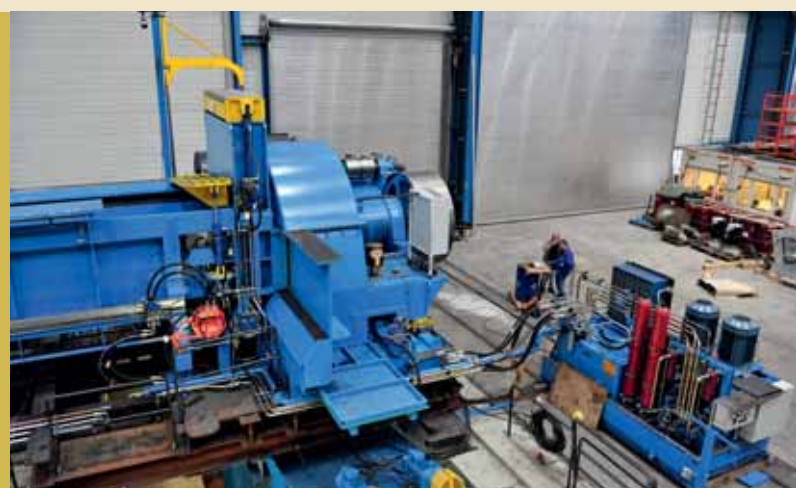
The hydraulic aggregate operates with 2 x 110 kW
