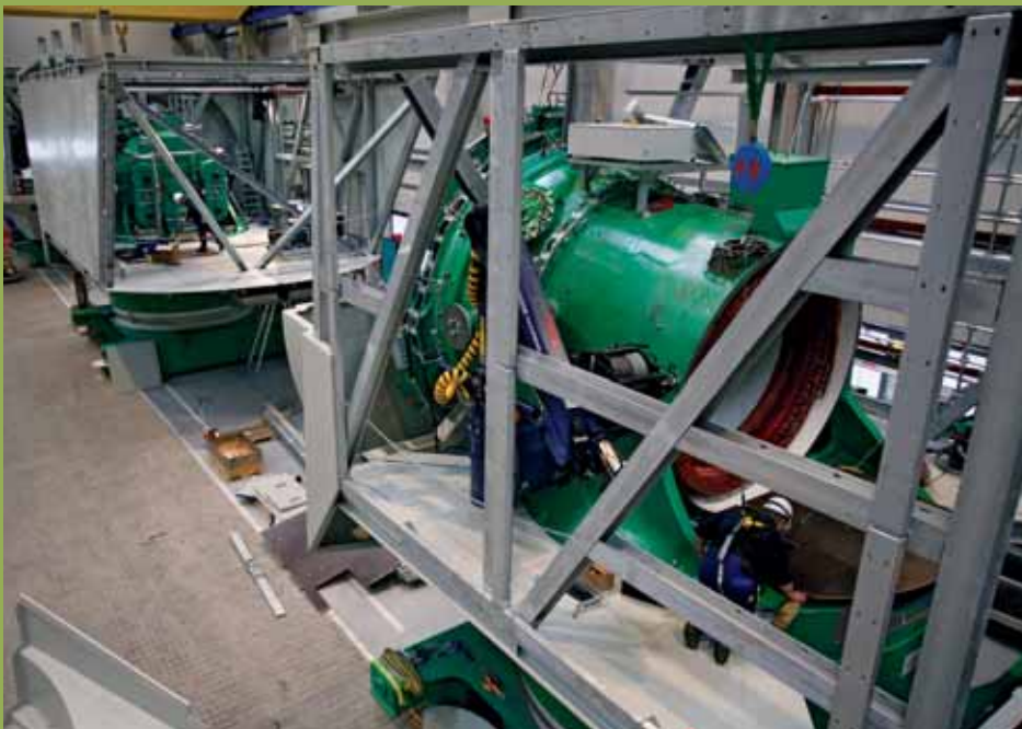
Machine carrier and lower deck in the Areva Wind final assembly hall (photo: Areva Wind)
