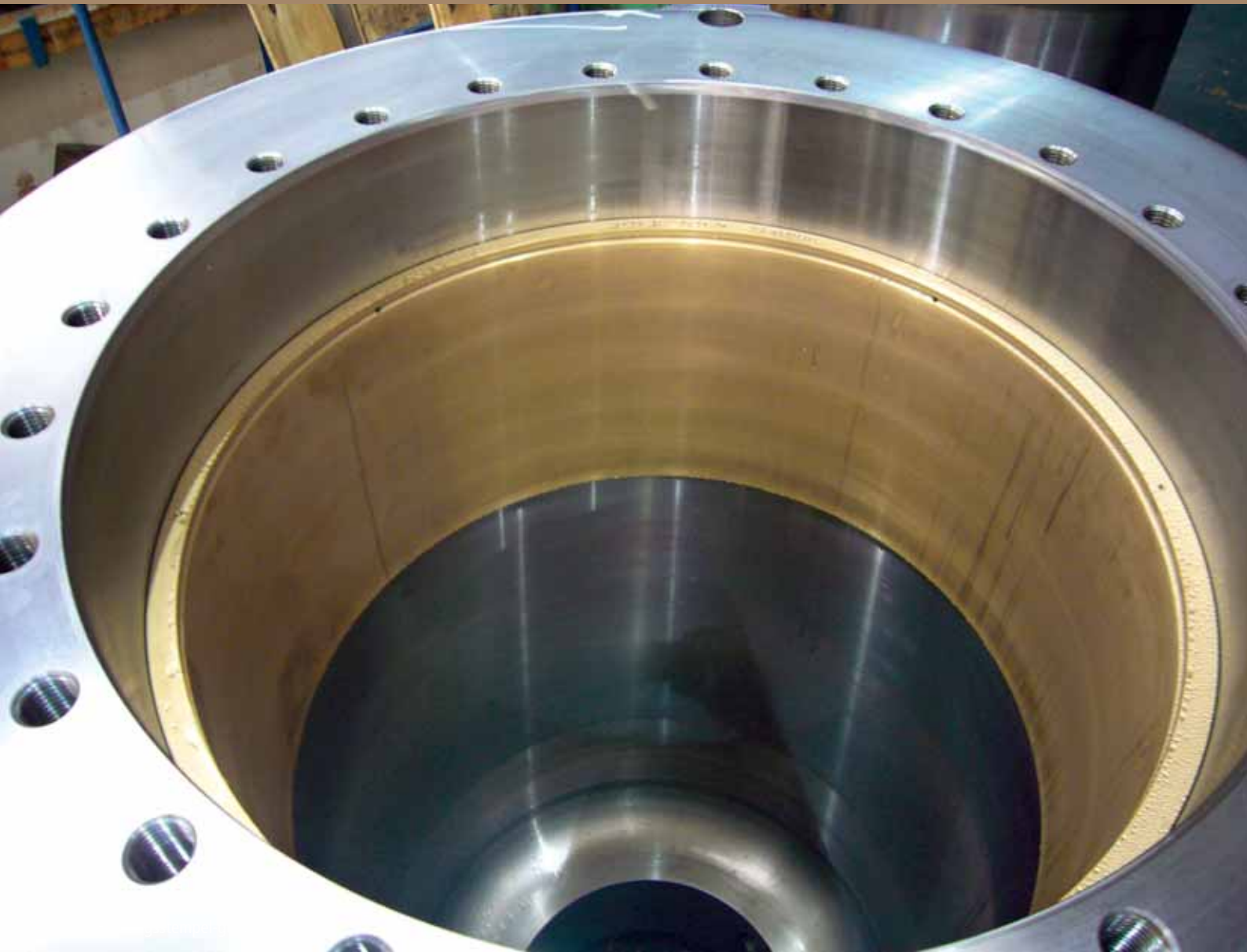
Main cylinder with bushing – in-house production
