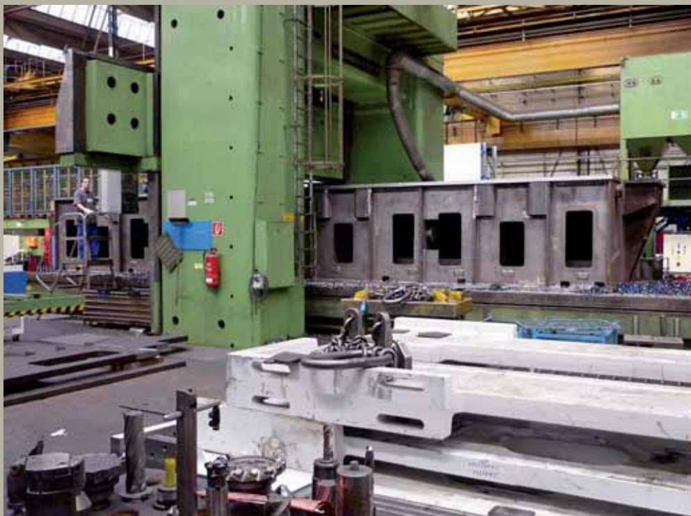
Lower beam during machining
