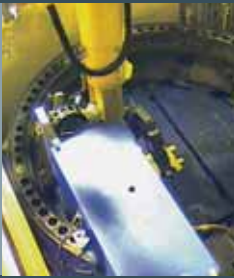
Segmentation of the RPV flange ring on a band saw
