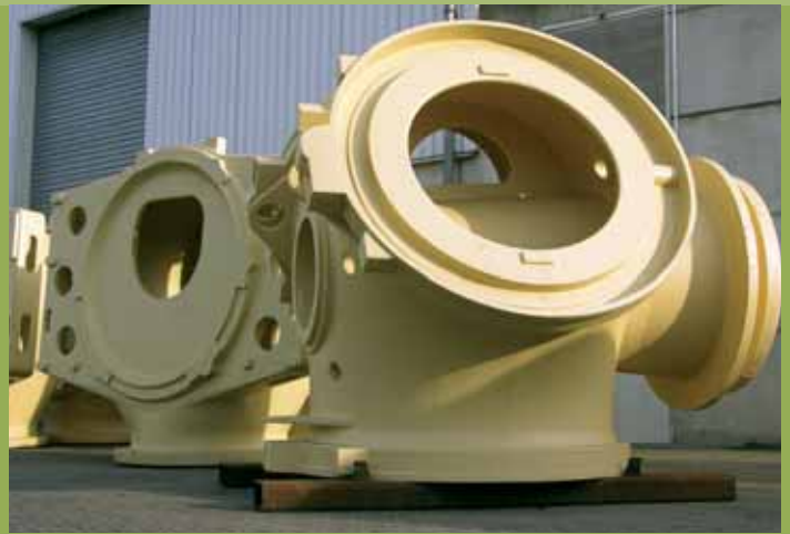
Rotor hub and machine carrier waiting for transportation
