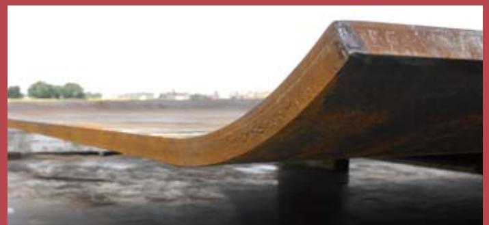
Bent plate for acceptance at Siempelkamp
