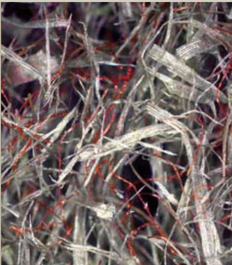
Homogeneous mixture of two-component binding fibers and wood fibers
