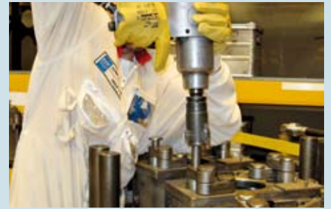
Electrical inspection of the rotary drive for the nuts
