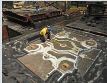
Molding of a plastics injection molding machine plate – to the left in the background the finished cope flask
