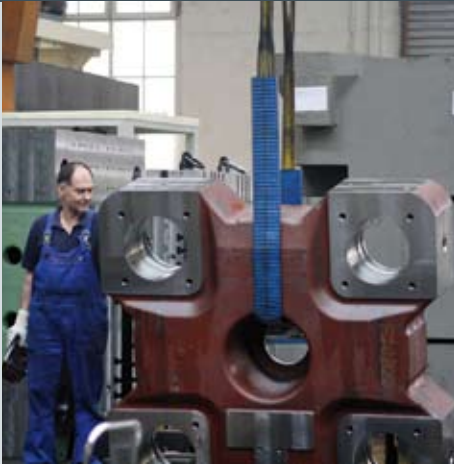
Assembly of a plastics injection molding machine (Source: KraussMaffei)
