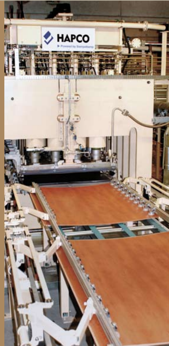
The short-cycle press from Hapco, powered by Siempelkamp
