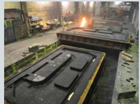
Prior to the casting process: combining of the cope and drag flask
