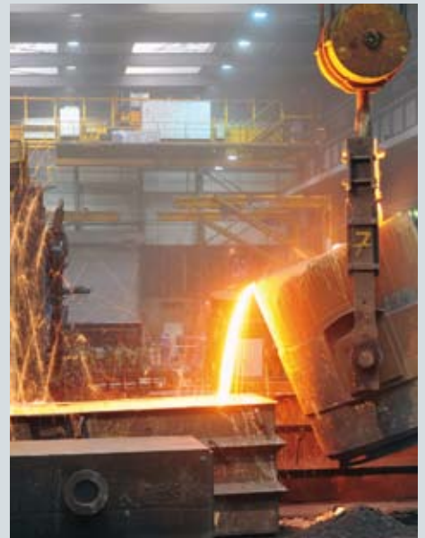
Casting of a cast iron plate
