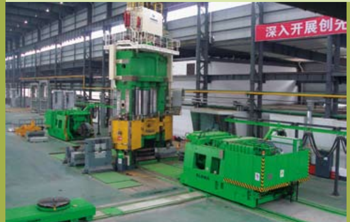
The complete unit: press, 2 manipulators, and the transport trolley
