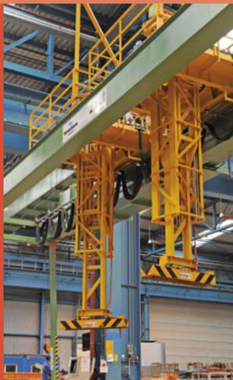
Double-girder bridge crane with rotatable trolley for loading the laser center
