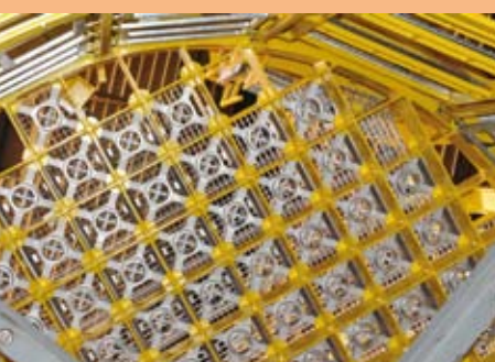
View from below the welded construction of the support ring for the lifting device for FA 3
