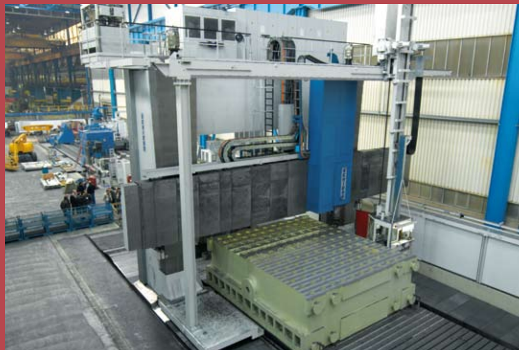
Machining of the beam at Siempelkamp
