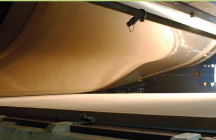
ContiRoll® infeed particleboard production
