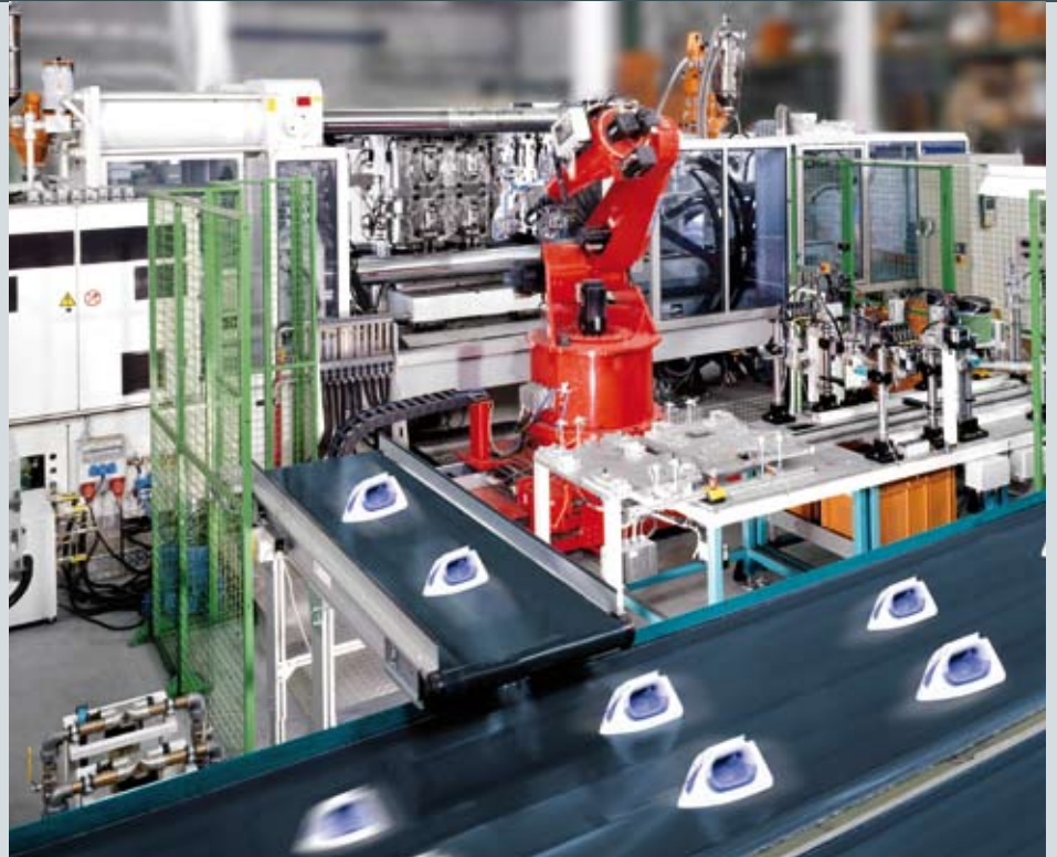
Production of iron housings (Source: KraussMaffei)
