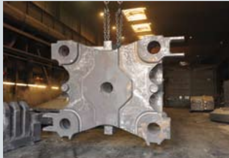
Finished cast iron plate prior to sand blasting
