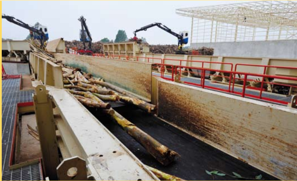
Log feed to the chipper
