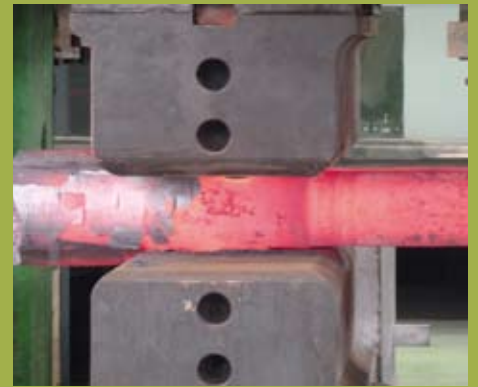
Forming process with special tools
