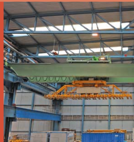
Double-girder bridge crane with rotatable trolley for loading the laser center
