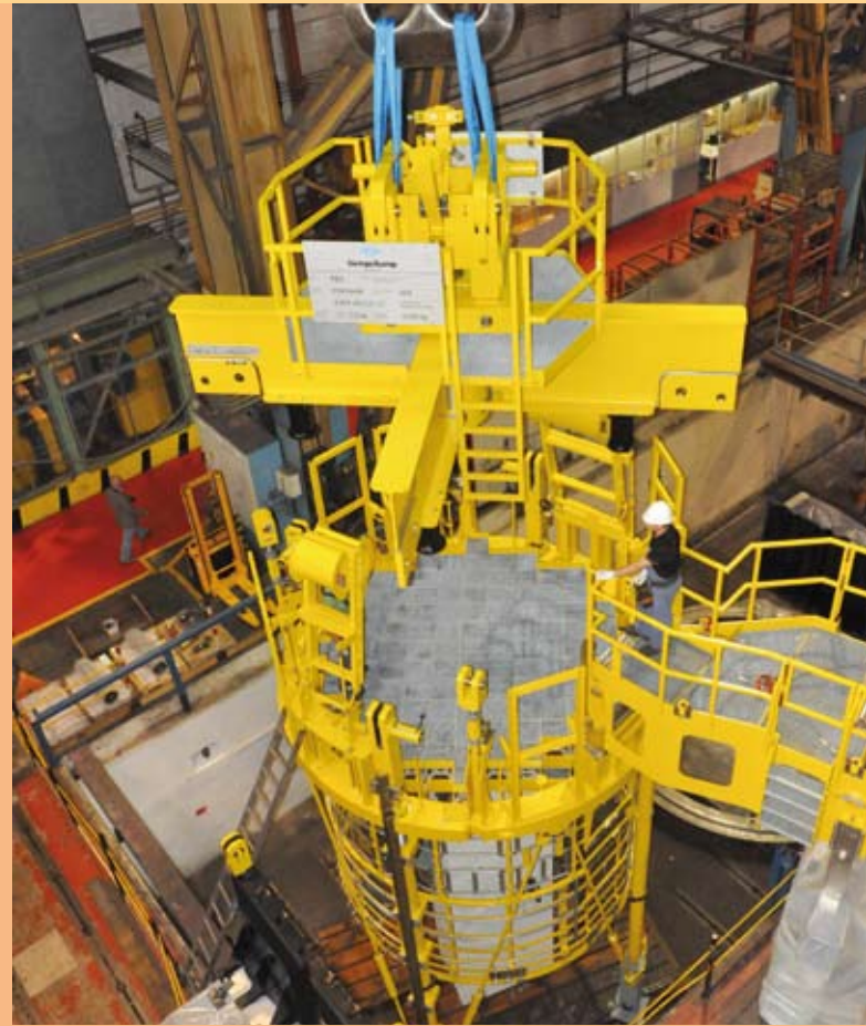
Lifting device for reactor pressure vessel closure head for Flamanville 3 on the test bench
