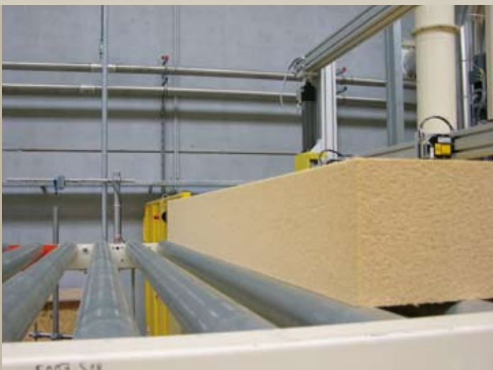
Wood-fiber insulation board manufactured according to the Siempelkamp dry-process
