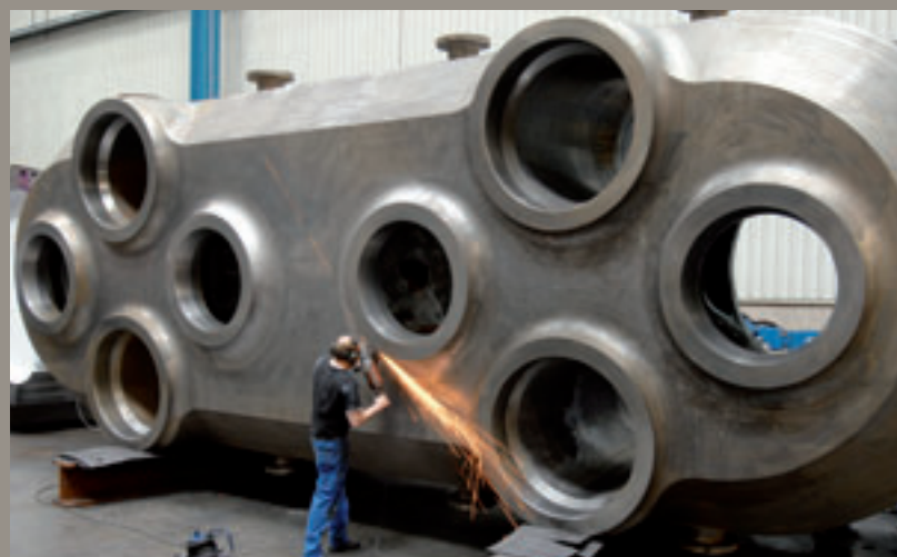
A stationary crosshead during final machining
