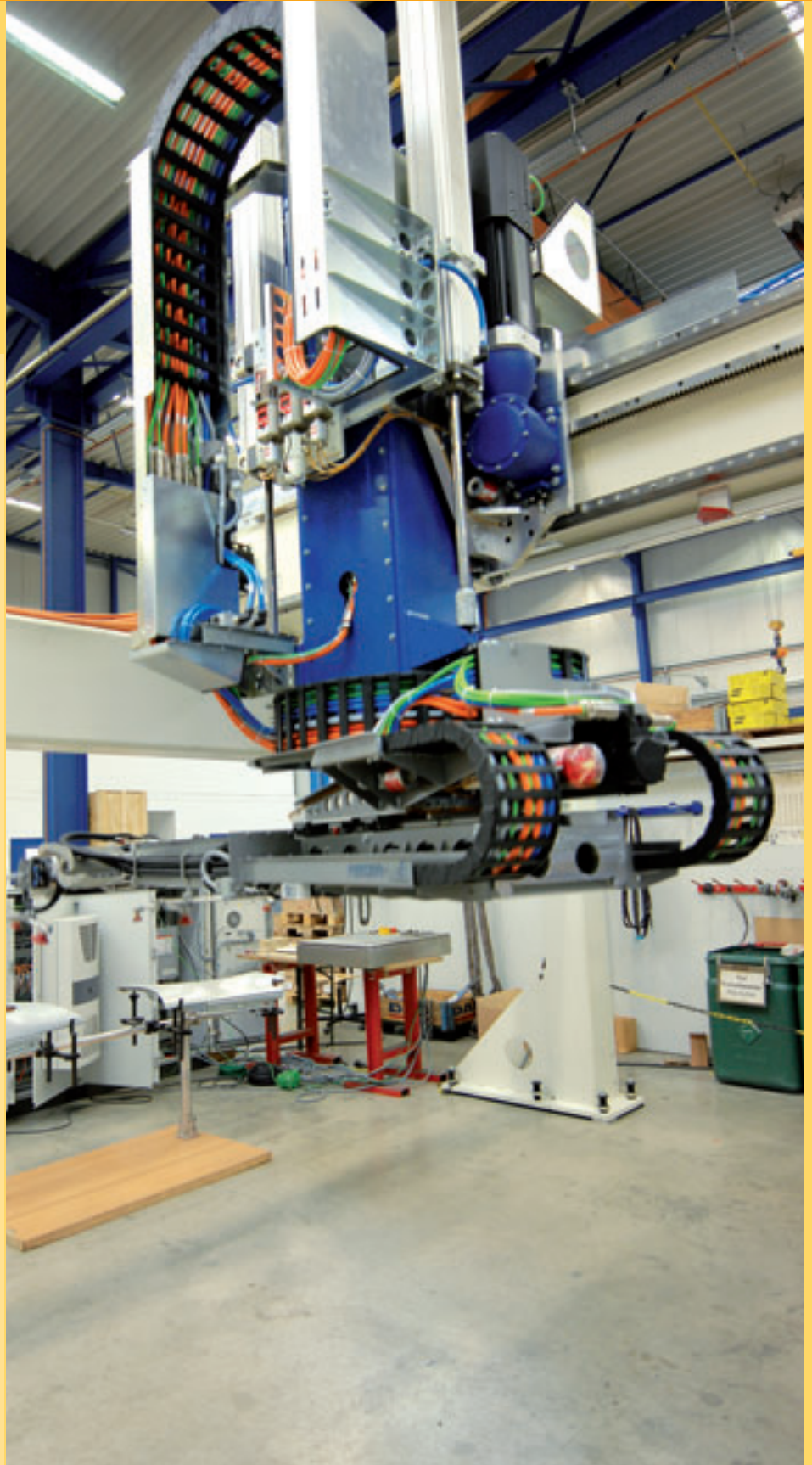
FEEDERplus8 in the endurance test
