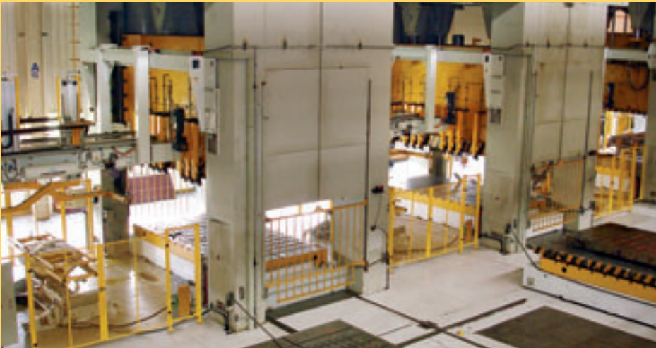
Press-to-press transfer with Strothmann feeders
