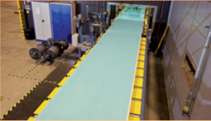
Automatic feeding of sealing strips
