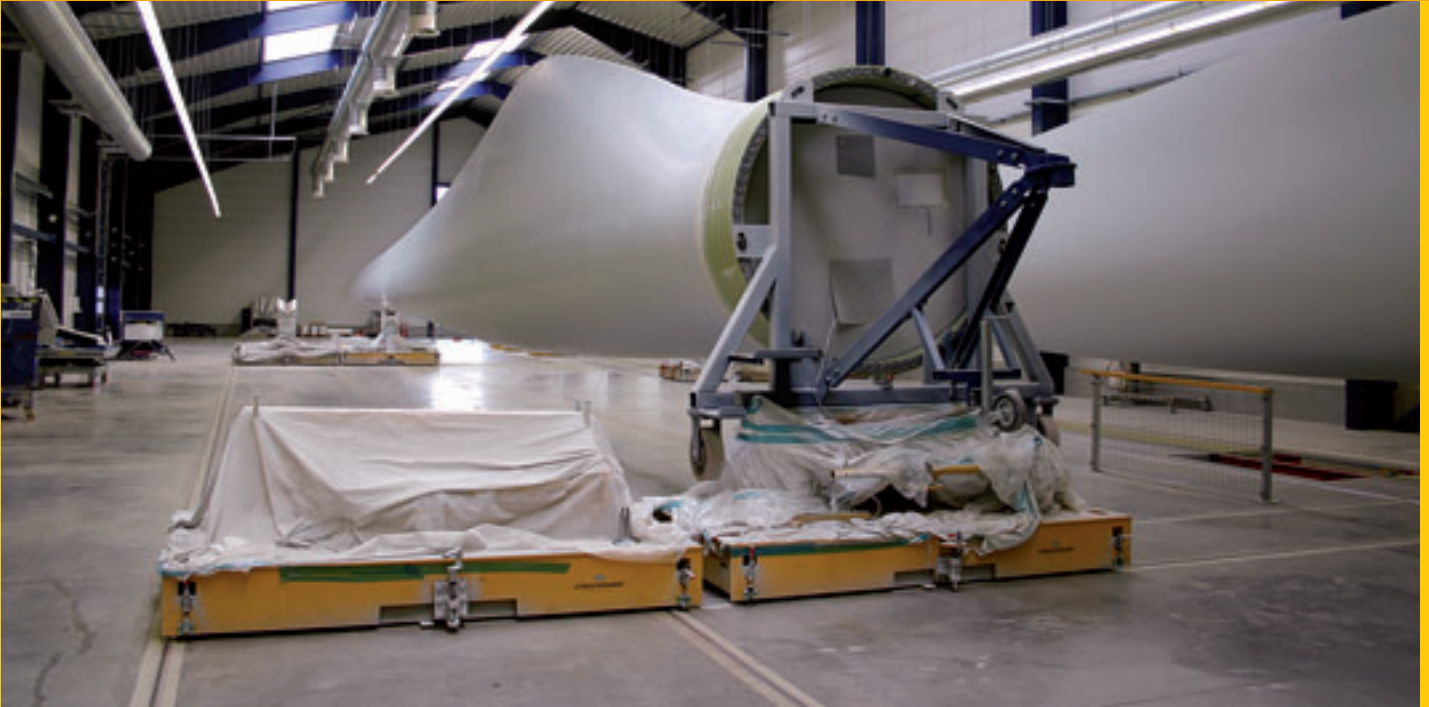
RoundTrack® and moving platforms during the manufacture of rotor blades
