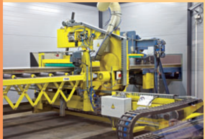
Band saw for cutting of the panels to length
