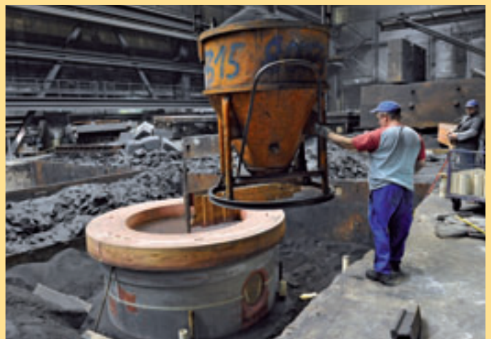
Pattern of a trunnion during molding
