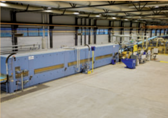
The double belt press: the core machine of the plant
