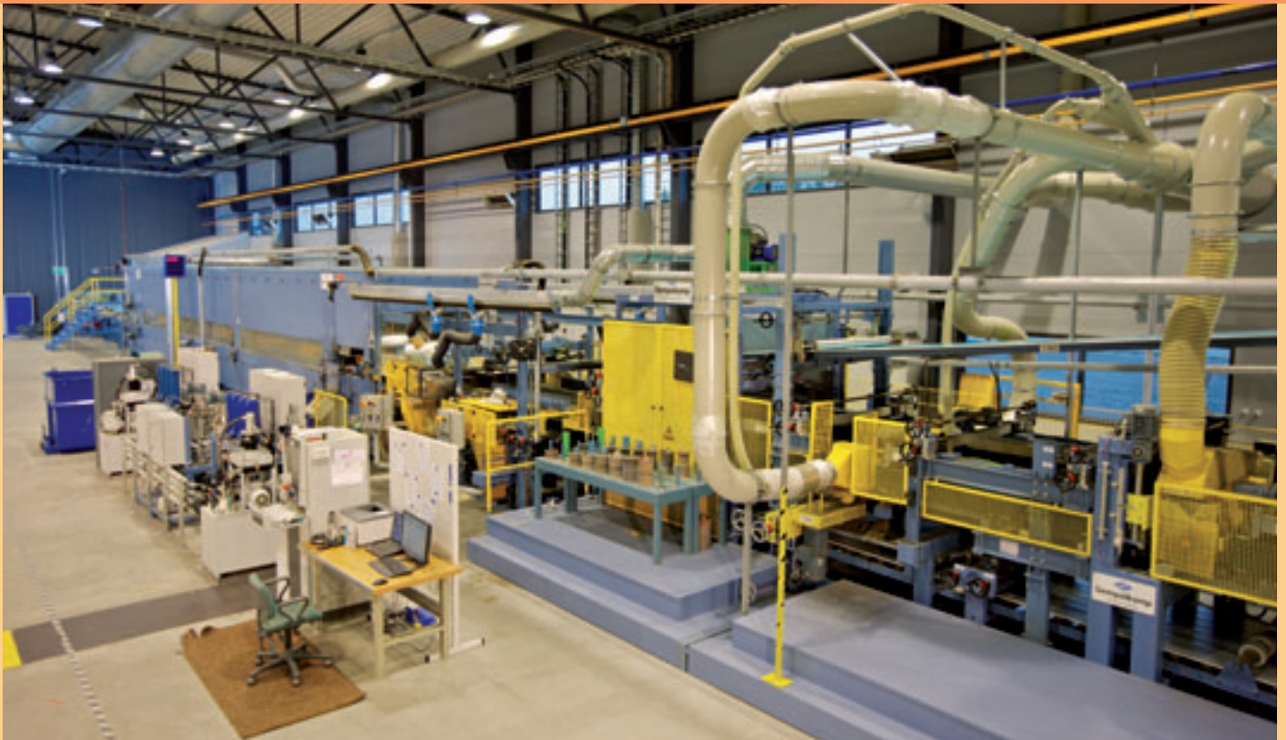
Glue application and joining of mineral wool core and cover layers
