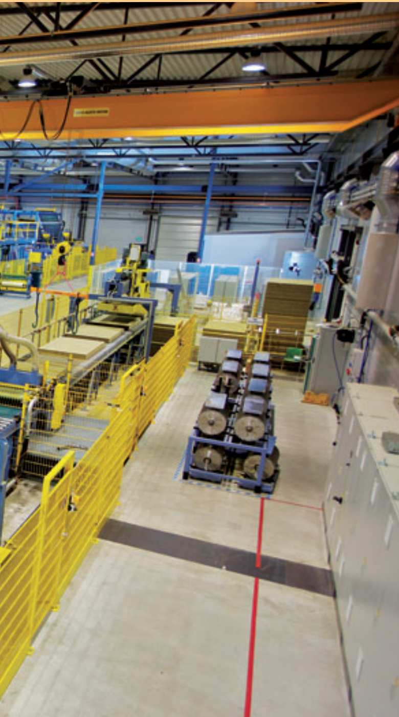
Cutting and automatic feeding of mineral wool strips
