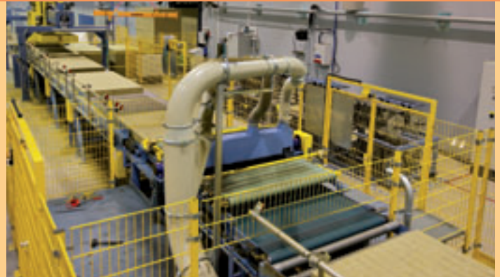
Automatic strip cutting of mineral wool boards
