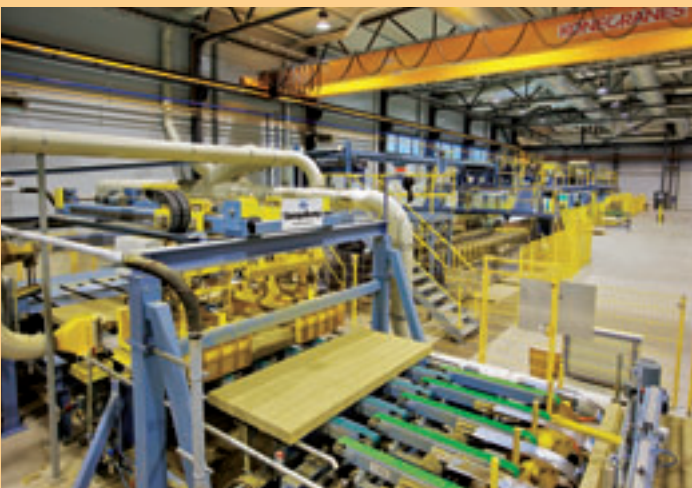
Strip trimming to control the tolerances
