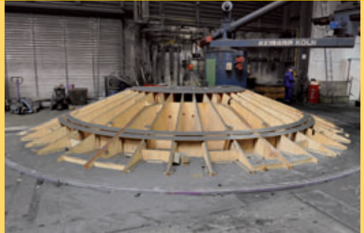
Wooden pattern of a 180° mill head segment
