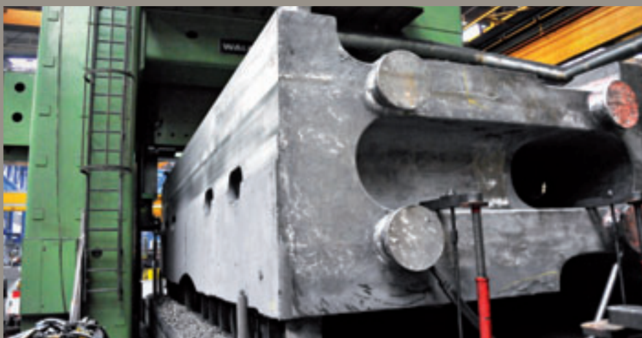
Machining of a segment on the Waldrich
