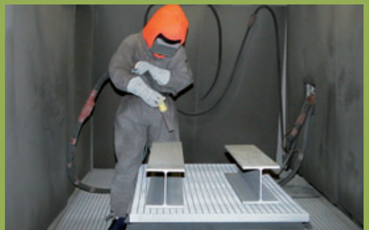
Decontamination using steel-grit blasting for a targeted surface abrasion
