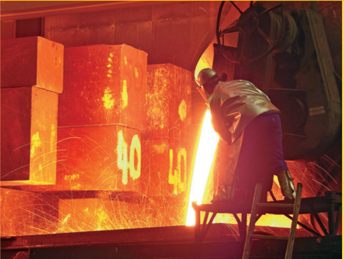
Casting of a mill head
