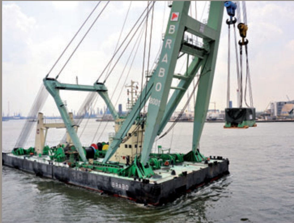
Loading with a pontoon crane
