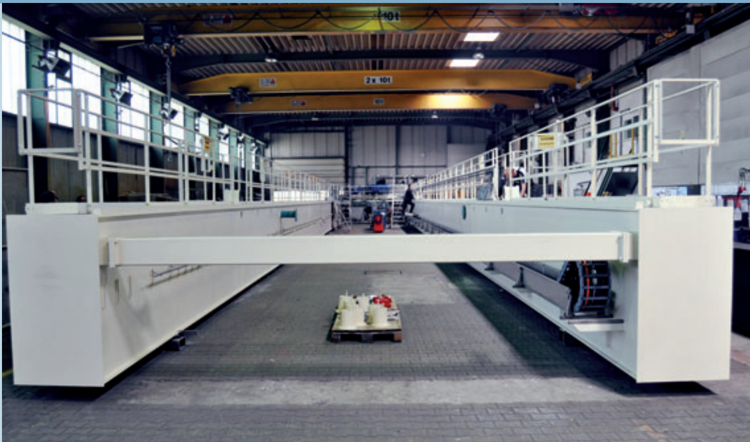
The finished crane system prior to acceptance by Siempelkamp Krantechnik
