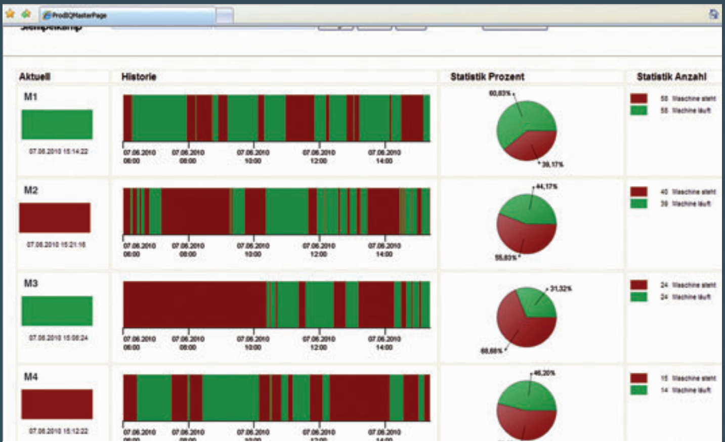
Machine run-time collection via Prod-IQ®
