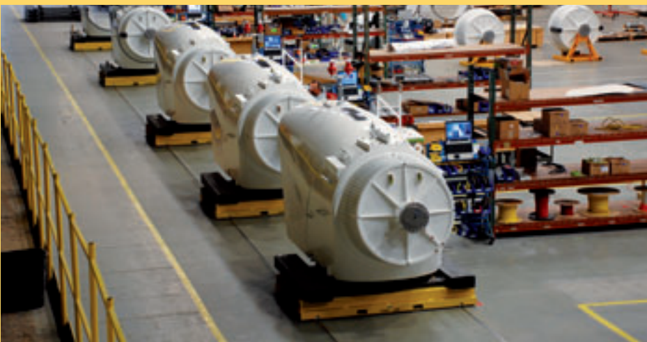
Continuous flow production with RoundTrack®
