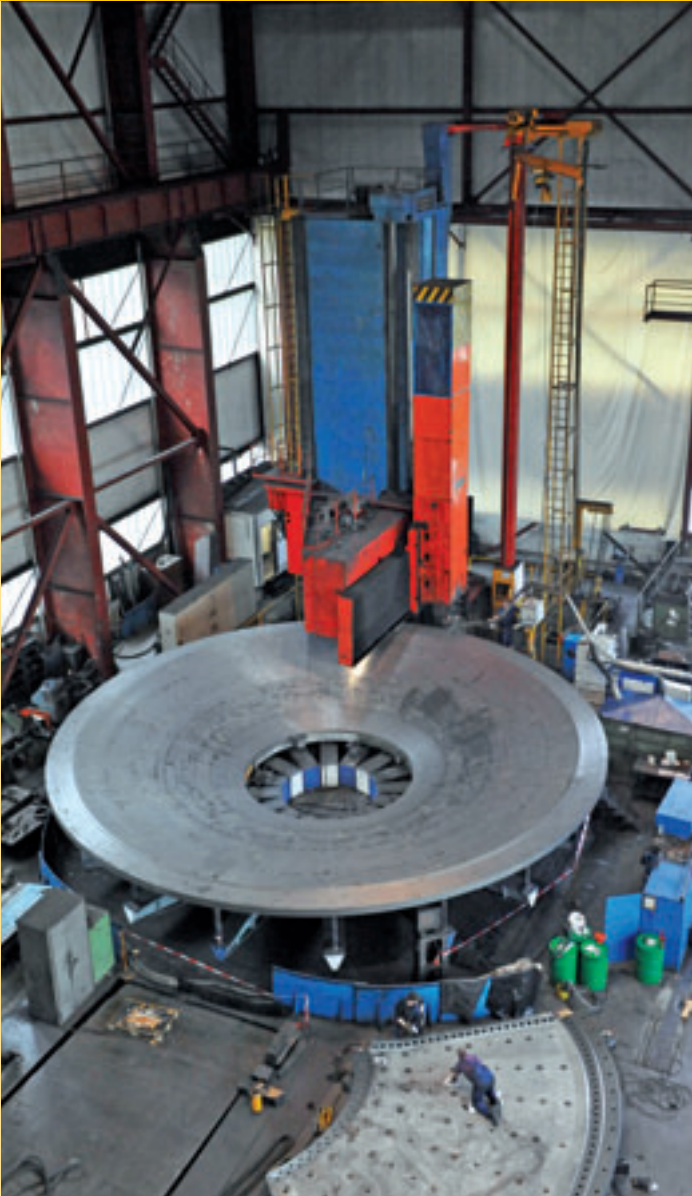
Mechanical machining – mill head on a vertical boring and turning mill
