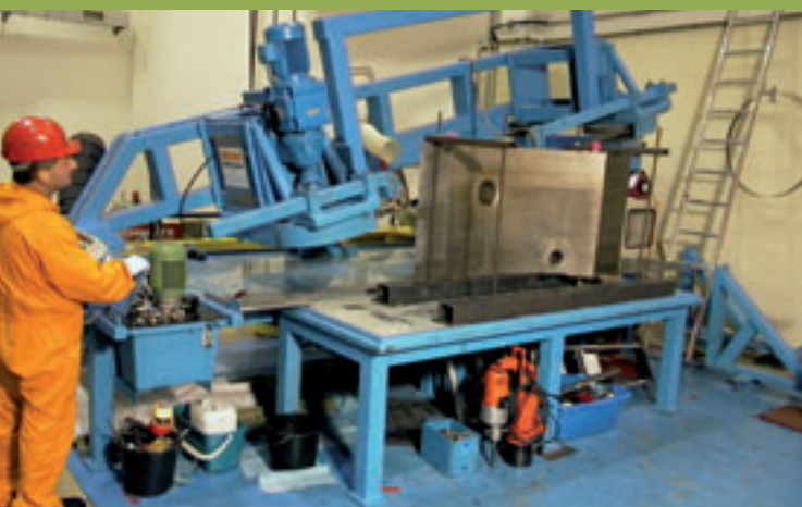
Heavy-walled steel parts are cut with a band saw
