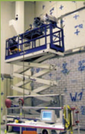
On-site release measurements of the building structure
