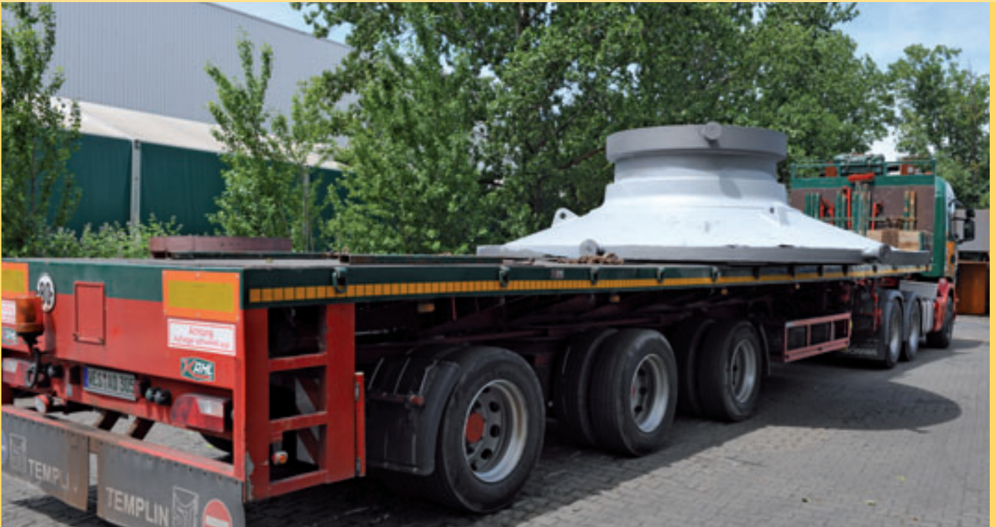
Mill head with trunnion on its way to the mechanical machining
