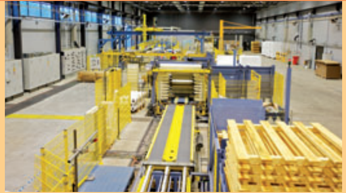
Packing line for panel stacks
